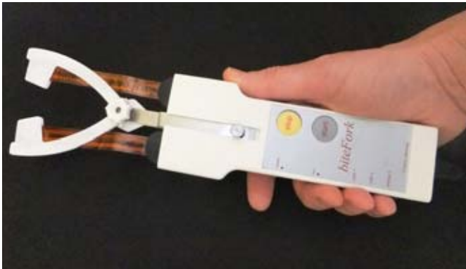
Fig 1 Handpiece of the biteForce System (Vi.me.S.).
